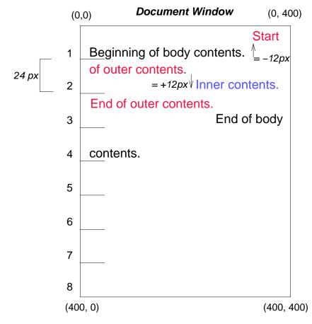
Note also that had the offset of *outer* been '-24px', the text of *outer* and the body text would have overlapped.
