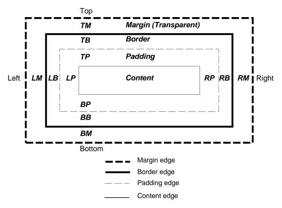
The margin, border, and padding can be broken down into top, right, bottom, and left segments (e.g., in the diagram, "LM" for left margin, "RP" for right padding, "TB" for top border, etc.).
