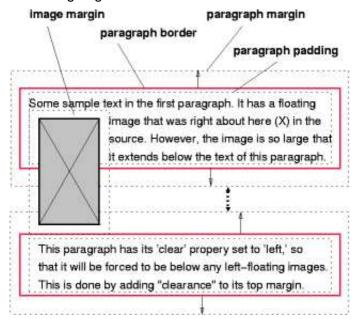
Both paragraphs have set 'clear: left', which causes the second paragraph to be "pushed down" to a position below the float —"clearance" is added above its top margin to accomplish this (see the 'clear' property).
