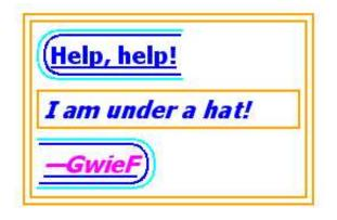
This diagram shows the boxes involved in the example above. The rounded aqua line represents the anonymous inline element wrapping the inline contents of the paragraph element, the rounded blue line represents the span element, and the orange lines represent the blocks.
